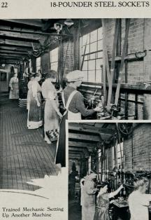
Milling Inside Thread of Steel Sockets for 18-Pounder Shrapnel Shells
