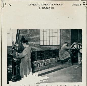
Screwing in the Base Plate and Rivetting ditto, 18-pounder High Explosive Shells
